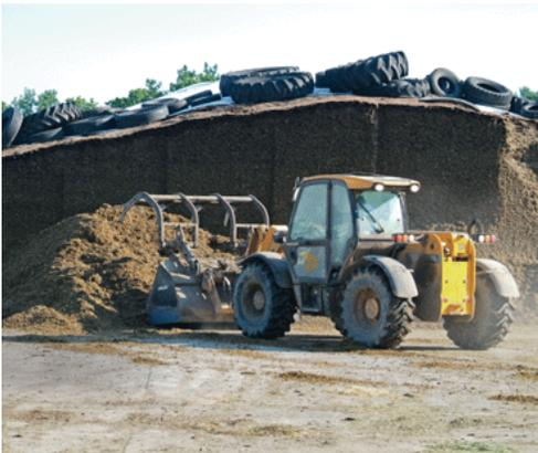
rule of thumb of 800 lbs of packing weight per ton of forage per hour was developed, again as a minimum.
