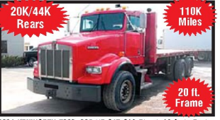
20K/44K Rears 110K Miles 20 ft. Frame 2004 KENWORTH T800; 335 HP CAT C10 Diesel; 10-Spd.; Engine Brake; Hendrickson Susp.; 22" Length X 102" Width; 5.29 Ratio; 22.5 Tires; All Steel Wheels; 240" WB; Tandem Axle; 20,000# F/A; 44,000# Full Locking Rears; Low Mile, Double Frame Flatbed Truck w/PTO; Will Separate Flatbed From Chassis; 20" Frame Behind Cab; 160" CT; 75% Rubber; 110,825 Miles; Stk. #4952 - $44,600
