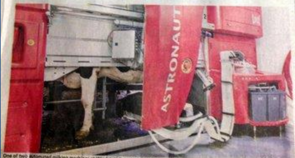
One of two automated milking machines at Windstett Farm in Genoa. The automated arm center uses lasers to guide and connect to
