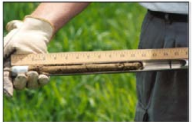
Figure 1: PSNT samples need to be taken over 12-inch depth when the corn is 6-12 inches tall to provide an accurate prediction of nitrate availability from organic N. http://nmsp.cals.cornell.edu/publications/factsheets/factsheet3.pdf
