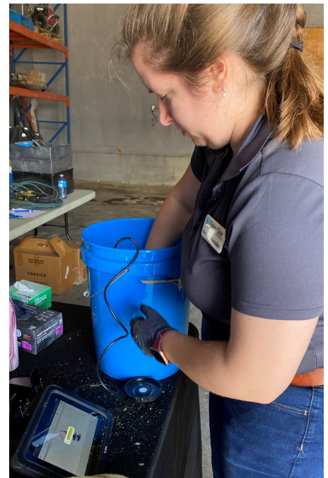
Sarah Fessenden from Dairy One using Near Infra-red technology to determine dry matter and starch content of corn silage samples at the 2022 Corn Silage Regional Dry Down Day.
