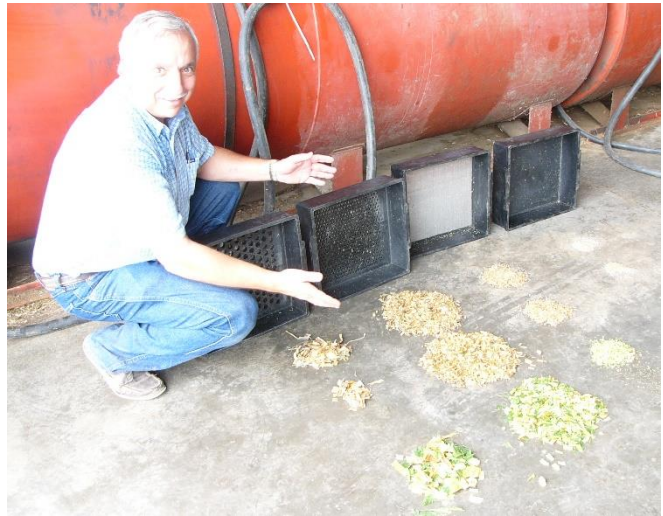
Regional dairy specialist Dave Balbian demonstrates the use of the Penn State Particle Separator to determine if corn silage is chopped to the proper length.
