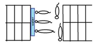
Diagram of a properly placed water trough in a crossover alley. The alley is wide enough to allow cows access to the trough while other cows are walking behind them.
