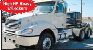
2007 Freightliner Columbia Daycab CAT 475 HP, Jakes, 15-Spd., 14,600# w/ 46,000# FULL LOCKING, Double Frame, 400,000 Miles
