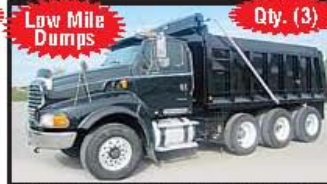
(3) 2005 Sterling, 14L Detroit 515 HP, Jakes, 230,000 Miles, 8LL Trans., Haulmax Susp., 24.5 Tires, Alum./Steel Wheels, 210" W.B., Tri-Axle, 18,000# F/A, 46,000# R/A, 16' Length Steel Body - $54,900 Each
