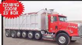
2000 Freightliner FLD; CAT C12 380 HP; Eng. Brake; Eaton Fuller 8LL; Air Lift 3rd, 4th, 5th, 6th; 4 Steerable; Dbl. Frame; Haul Max Susp.; 20K FA; 46K RA; 295" W.B.; Alum. Wheels; Alfab 23' Alum. Box
