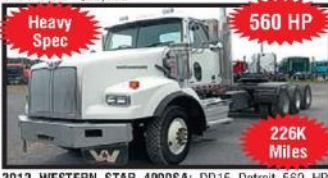
2012 WESTERN STAR 4900SA: DD15 Detroit 560 HP; 18-Spd.; Tri-Axle; 4.30 Ratio; 24.5 Tires; Alum./Steel Wheels; 260" WB; 20,000# F/A; 69,000# Full Locking Rears; Tri-Drive Or Drop Axle To Make Long Chassis - Your Choice; Double Framed; 310" Bridge Measurement; 23" Frame Behind Cab; 226,769 Miles; Stk. #5426 - $56,900
