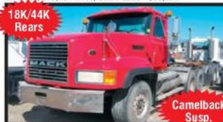
1998 MACK CL713: 460 HP E7 Diesel; 9-Spd. Trans.; Tandem Axle; 22.5 Tires; Spoke Wheels; 169" WB; 18,000# F/A; 44,000# R/A; Heavy Spec, Double Frame daycab w/Wetline System; EXPORTERS WELCOME. WE DELIVER TO ALL US & FOREIGN PORTS; 152,953 Miles; Stk. #5367 - $24,500
