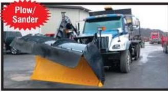
2006 INTERNATIONAL 7500: 300 HP Int'l HT570; Allison Auto. Trans.; Tandem Axle; 22.5 Tires; Alum./Steel Wheels; 190" WB; 18,000# F/A; 46,000# R/A; Plow/Sander Truck w/Stainless Steel Trench 12-Cu. Yd. Spreader w/Backup John Controls & 12" Trench Plow & Wing; ASK FOR MUNICIPAL PRICING! ; 213,391 Miles; Stk. #5292 - $39,900
