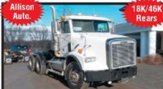
2002 FREIGHTLINER FLD112: 370 HP Cummins ISM; Allison Auto. Trans.; Tandem Axle; 4.89 Ratio; 315/80R22.5 Tires; All Steel Wheels; 170" WB; 16,000# F/A; 46,000# R/A; Double Frame Tractor w/Wetline System; 306,867 Miles; Stk. #5297 - $29,900
