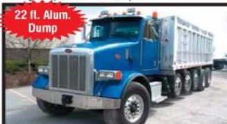
2001 PETERBILT 357: 425 HP CAT C12; 8LL Trans.; Five Axle; Engine Brake; 22.5 Tires; Alum. Wheels; 290" WB; 18,000# F/A; 46,000# Full Locking Rears; 6-Axle Dump Truck w/Double Frame; (3) Steerable 9,000# Lift Axles; 22" Alum. Box w/64" Sides; 842,267 Miles; Stk. #5346 - $54,900
