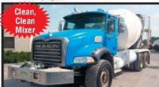
2005 MACK GRANITE CT713: 330 HP Mack; 9-Spd.; 22.5 Tires; 210" WB; 20,000# F/A; 44,000# R/A; Clean, Double Frame 10 Cu. Yd. Mixer; 18" Frame Behind Cab; 148" CT; 103,479 Miles; Stk. #5583 - $59,900
