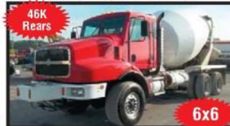
(QTY 3) 2006 OSHKOSH F2346 6X6: 320 HP Cummins ISM; 10-Spd.; Tandem Axle; Color: Red; 22.5 Tires; Alum./Steel Wheels; 211" WB; 23,000# F/A; 45,000# Full Locking Rears; 10 1/2 Cu. Yd. McNeilus Mixer; 19' Frame Behind Cab; 152" CT; 139,840 Miles; Stk. #5580/5581/5582 - $44,900 EACH
