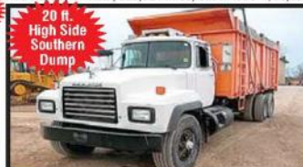
1997 MACK RD690S: 300 HP Mack E7; 10-Spd.; 20' Steel Box; 22.5 Tires; Spoke Wheels; 250" WB; 18,000# F/A; 44,000# R/A; Double Frame; Box Has High Side, Divider & Tarp; 147,222 Miles; Sk. #5312 - $32,500
