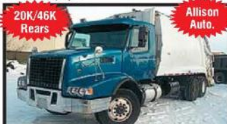
2004 VOLVO VHD648200: 395 HP Volvo VED12; Engine Brake; Allison HD4560P 6-Spd. Auto. Trans.; Tandem Axle; 4.89 Ratio; 315/80R22.5 Tires; All Steel Wheels; 228" WB; 20,000# F/A; 46,000# Full Locking Rears, Double Frame; 25 Cu. Yd. McNeilus Packer; 371,577 Miles; Sk. #5676 - $27,250
