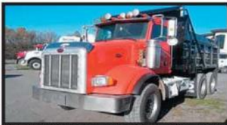
2006 PETERBILT 378: C15 Cat 475 HP; 18-Spd.; Tandem Axle; Engine Brake; 24.5 Tires; Alum. Wheels; 188" WB; 20,000# F/A; 46,000# Full Locking R/A; Double Frame; 14' Steel Body; Tarp; Hitch; 434,815 Mi.; Sk. #5610 - $49,900
