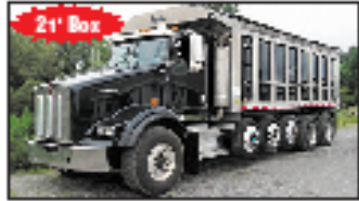
2007 Kenworth T800, CAT C13, 430 h.p., 8LL, ang. brake, 21' alum. box, Chalmers susp., 288" wb, alu./steel wheels, 20,000# FIA, 46,000# FIA, 114,000 miles, 5 axle dump $62,900.
