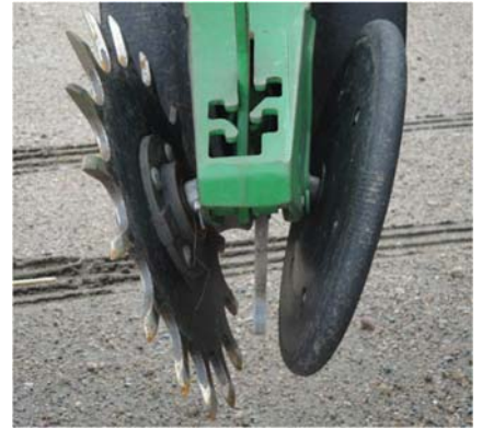
Figure 2. By replacing one solid closing wheel with a spiked one, closing the seed-vee becomes easier in a variety of conditions. The spiked wheel fractures the sidewall and provides some loose soil while the solid one provides some seed firming and depth control. (If the closing wheels can be staggered, mount the spiked one in front.)
