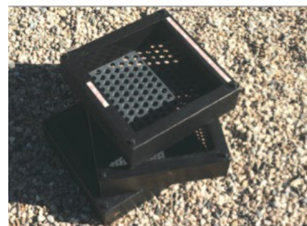
Figure 1. Penn State Particle Size Separator. The two screens are offset to show the diameter of the holes.
