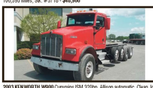
2003 KENWORTH W900 Cummins ISM 320hp, Allison automatic, Clean, low mile cab and chassis with 20k front axle, (2) 11k steerable lift aides, 44k full locking rears on Chalmers suspension, 5.43 ratio, 250" wheelbase, 21" of frame behind the cab, 156" C-T Muffler takes up 12" behind the cab. Stk #6016 - $54,900
