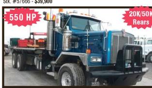
550 HP 20K/50K Rears 2005 KENWORTH C500B; 550 HP CAT C15; 20,000# F/A; 50,000# R/A; Chalmers Susp.; 4.89 Ratio; 24.5 Tires; 272" WB; Tulsa Rulmek Winch; 17' x 9' Deck w/Tail-Roller; 21" Frame Behind Cab; 192" CT; 343,792 Miles; Stk. #5911 - $49,500
