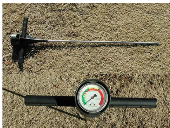
Figure 3. Soil penetrometer (Compaction meter)
