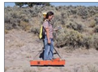
Figure 1: The Geonics EM38-MK2 soil electrical conductivity meter. http://www.geonics.com/
