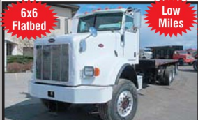
6x6 Flatbed 2005 PETERBILT 357 6x6; Clean Double Frame 24'6" Flatbed Truck; CAT 350 HP; 8LL Trans.; 22K F/A; 46K Full Locking Rears; 425/65R22.5 Tires; Hendrickson Haulmax Susp.; 5.65 Ratio; 288" WB; 218" CT; 30' Frame Behind Cab; Will Separate Bed from Chassis; 174,108 Miles; Stk. #5701 - $49,900
