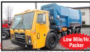
2012 MACK LEU613 PACKER: Double Frame; Labrie Side Load Packer; 20K F/A; 46K Rears; Haulmax Susp.; Allison Auto. Trans.; LH/RH Side Drives; 212" WB; 180" CT; 206" Frame Behind Cab if the Packer is Removed. ***HP Can Be Increased to 395-425 with Software Flash***; 59,375 Miles/13,276 Hours - $48,850
