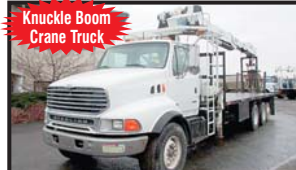
2002 STERLING LT9500 CRANE TRUCK: w/MT24562 Knuckle Boom Crane; 350 HP Cummins ISM; 8L Trans.; 82" Reach; 5,000 lbs. Lift Capacity; 24" Steel Flatbed; 20K F/A; 46K Full Locking Rears; Stearley Lift Axle; T-Ride Susp.; 270" WB; 30" Frame Behind Cab; 208" CT; 181,865 Miles; Stk. # 6750 - $51,900
