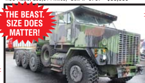
2000 OSHKOSH: Detroit Diesel V8 500 HP Turbo Diesel Engine; Engine Brake; Automatic Trans.; 86,000 lb. GVWR; Two 5,000 lb. Winches; Aux. Winch; 8x8; Rear Wheel Steer; Exhaust Brake; Air Ride Susp.; PTO; Fifth Wheel Ramp Plates; Central Tire Inflation System; Stk. # 6695 - $88,900
