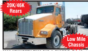
2009 KENWORTH T800 CAB & CHASSIS ; Clean Double Frame; 355 HP Cummins ISM (Can Be Re-Rated To 425 HP); 18-Spd. Manual; 264" WB; 21" Frame Behind Cab; 186" CT; 20K F/A; 46K Full Locking Rears On Neway Air Ride; 4,30 Ratio; PTO w/Controls; 107,210 Miles; Stk. # 6778 - $54,900
