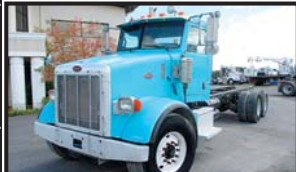
2006 PETERBILT 357 CAB & CHASSIS ; 335 HP CAT C11; Allison Auto. Trans.; 20K F/A; 46K Locking Rears; Chalmers Susp.; 254" WB; 170" CT; 21" 6" Frame Behind Cab; 205,344 Miles; Stk. # 6822 - $56,900
