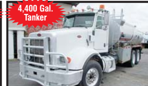
2008 PETERBILT 365 TANK TRUCK ; Double Frame w/4,400 Gal. Steel Tank; Cummins 410 HP; 13-Spd.; 14.6K F/A; 44K Full Locking Rears on Air Trac Susp.; 228" WB; 156" CT; 21" Frame Behind Cab; PTO; 529,094 Miles; Stk. # 6857 - $44,900
