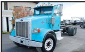
2006 PETERBILT 357 CAB & CHASSIS ; 335 HP CAT C11; Allison Auto. Trans.; 20K F/A; 46K Locking Rears; Chalmers Susp.; 254" WB; 170" CT; 21" Frame Behind Cab; 205,344 Miles; Stk. # 6822 - $56,900
