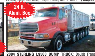
2004 STERLING L9500 DUMP TRUCK ; Double Frame; Mercedes OM 460LA 18-Spd. Manual; 24" Allfab Alum. Body w/60" Sides and 6" Sideboards; Tarp; 20K F/A; 46K Locking Rears; Hendrickson HN Susp.; (4) 11K Steerable Lift Axles; 425/65R22.5 Front; 11R24.5 Drive Tires; 310" WB; 246" CVT; 24'6" Frame Behind Cab; 583,000 Miles; Stk. # 6931 - $69,900
