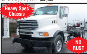
2007 STERLING L9500 CAB & CHASSIS ; Clean; Double Frame; 385 HP CAT C13; Allison Auto.; 20K F/A; 46K R/A; Hendrickson Spring Susp.; 248" WB; 184" CT; 21" Frame Behind Cab (Muffler Takes Up 14"); 276,988 Miles; Stk. # 6914 - $49,500
