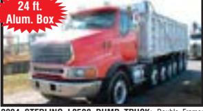
2004 FREIGHTLINER L9500 DUMP TRUCK: Double Frame; Mercedes OM 460LA 18-Spd. Manual; 24' All-Alum. Body w/60" Sides and 6" Sideboards; Tarp; 20K F/A; 46K Locking Rears; Hendrickson HN Susp.; (4) 11K Steerable Lift Axles; 425/65R22.5 Front; 11R24.5 Drive Tires; 310" WB; 246" CVT 24'6" Frame Behind Cab; 583,000 Miles; Stk. # 6931 - $62,900
