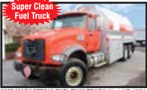
2007 MACK CTP713 FUEL TANK TRUCK: Mack MP-405M; Allison Auto. Trans.; Clean, Double Frame Fuel Truck w/Allied Manufacturing 4,700 Gal Fuel Tank; (5) Compartments; 18K F/A; 46K Rears; Air Ride Susp.; 274" WB; 182" CT; 23'6" Frame Behind Cab; 209,176 Miles; Stk. # 6916 - $64,500
