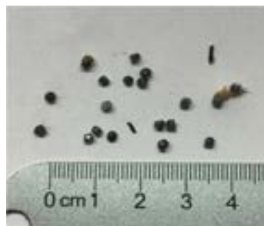
Figure 2: Birdshot and Other Metals Found at Further Processors (Source: Michaela Clowser, NCBA)
