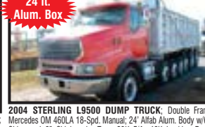
24 ft. Alum. Box 2004 STERLING L9500 DUMP TRUCK; Double Frame; Mercedes OM 460LA 18-Spd. Manual; 24" All-Alum. Body w/80" Sides and 6" Sideboards; Tarp; 20K F/A; 46K Locking Rears; Hendrickson HN Susp.; (4) 11K Steerable Lift Axles; 425/65R22.5 Front; 11R24.5 Drive Tires; 310" WB; 246" CVT/24'6" Frame Behind Cab; 583,000 Miles; Stk. # 6931 - $62,900
