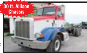
30 ft. Allison Chassis 2015 PETERBILT 365 CAB & CHASSIS; 455 HP Paccar MX13; Allison Auto. Trans.; Double Frame; 20K F/A; 46K Rears; Hendrickson Haulmax Susp.; 278" WB; 208" CTR; 30" Frame; Pintle Hook; Plumbed For Pup Trailer; 235,209 Miles; Stk. # 6952 - $68,500
