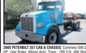
2005 PETERBILT 357 CAB & CHASSIS ; Cummins ISM 385 HP; Jake Brake; Allison Auto. Trans.; 20K F/A; 46K Rears; 252" WB; 21" Frame Behind Cab; 168" CT; Chalmers Susp.; Rear Engine PTO (REPTO); Frame Has Been Sandblasted and Painted; 68,882 Miles and 14,682 Hours; Stk. # 6924 - $76,900
