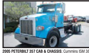
24 ft. Alum. Box 2005 PETERBILT 357 CAB & CHASSIS; Cummins ISM 385 HP; Jake Brake; Allison Auto. Trans.; 20K F/A; 46K Rears; 252" WB; 21" Frame Behind Cab; 168" CT; Chalmers Susp.; Rear Engine PTO (REPTO); Frame Has Been Sandblasted and Painted; 68,882 Miles and 14,682 Hours; Stk. # 6824 - $56,900
