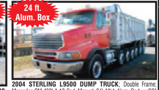
24 ft. Alum. Box 2004 STERLING L9500 DUMP TRUCK; Double Frame; Mercedes OM 460LA 18-Spd. Manual; 24" Allfab Alum. Body w/60" Sides and 6" Sideboards; Tarp; 20K F/A; 46K Locking Rears; Hendrickson HN Susp.; (4) 11K Steerable Lift Axles; 425/65R22.5 Front; 11R24.5 Drive Tires; 310" WB; 246" CVT; 24'6" Frame Behind Cab; 583,000 Miles; Stk. # 6931 - $62,900
