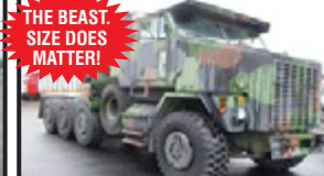
THE BEAST. SIZE DOES MATTER! 2000 OSHKOSH; Detroit Diesel V8 500 HP Turbo Diesel Engine; Engine Brake; Automatic Trans.; 86,000 lb. GVWR; Two 55,000 lb. Winches; Aux. Winch; 8x8; Rear Wheel Steer; Exhaust Brake; Air Ride Susp.; PTO; Fifth Wheel Ramp Plates; Central Tire Inflation System; Stk. # 6696 - $59,900
