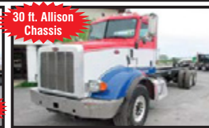
30 ft. Allison Chassis 2015 PETERBILT 365 CAB & CHASSIS; 455 HP Paccar MX13; Allison Auto. Trans.; Double Frame; 20K F/A; 46K Rears; Hendrickson Hauimaax Susp.; 278" WB; 208" CTR; 30" Frame; Pintle Hook; Plumbed For Pup Trailer; 295,209 Miles; Stk. # 6952 - $68,500
