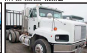
1999 INTERNATIONAL PAYSTAR 5000 DOUBLE FRAME DAYCAB ; Cummins N14 370+ HP; Allison Auto. Trans.; 18K F/A; NEWAY Air Ride Susp.; Wetline; Rubber 95%; 90,427 Miles; Stk. # 6745 - $34,900
