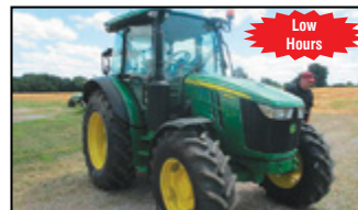
Low Hours 2019 JOHN DEERE 5090R; 3 Available, MFWD tractor 90hp, with low hours, new tires, 16F/16R power shuttle transmission, suspension cab, rider seat, full cab w/ heat/AC, 3 remotes. Some remaining factory warranty; 900-1200 Hrs. Stk. # 370 - $54,500
