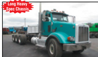
Long Heavy Spec Chassis 2014 PETERBILT 365 CAB & CHASSIS; TRI-DRIVE; 450 HP Cummins ISX; 18-Spd. Transmission; 20K F/A; 64K Triple Locking Rears; Air Trac Susp.; 445/65R22.5 Front, 11R24.5 Rear Tires; 278" WB; 334" Bridge; 24" Frame Behind Cab, PTO, 168,725 Miles; Stk. # 7020 - $57,000 EACH
