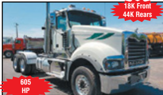
2015 MACK TITAN T0713: Mack MP10-605C 605 HP Fuller 18 speed transmission, headcack rack, 18K front 44K rears with diff. lock, air ride suspension; 222" wb, dual exhaust air cleaners, wet line. 400,130 miles; Sk. # 7082 - $73,500
