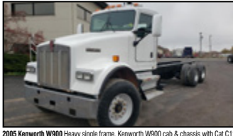
2005 Kenworth W900 Heavy single frame, Kenworth W900 cab & chassis with Cat C11 engine with 350 HP Eaton-Fuller 8L transmission, 20K front axle, 46K full locking rears, Allison automatic, 250" wb, 21' 10" of frame, 160" C-T (muffler takes 1' of these measurements) 20K front, 46K locking rear, rear engine PTO (REPTO) 187,683 miles; Sk. # 7085 - $52,900
