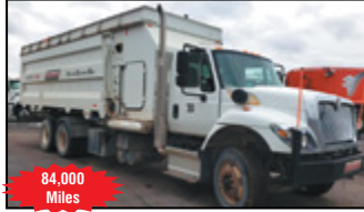
2018 INTERNATIONAL WORKSTAR 7400 DOUBLE FRAMED DELIVERY TRUCK with Rot-Max 1102-23 RDB (Roll-Over Delivery Box), Cummins 350 HP, Allison Auto. Trans.; 20K F/A; 46K R/A; Haulmax Susp.; 250" WB; 182" CT; 26" Frame Behind Cab; 10'8" High/12" High w/Extensions; Sk. # 7032 - $65,800
