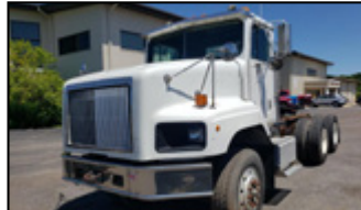
1999 International Paystar 5600 Double frame day cab with 184" wheelbase, Allison HT 750 DR automatic transmission, 12,350 lb. front axle, 42,400 lb. rears, NEWAY air ride, wet line, rubber 95%, 1666,030 miles, sk. # 6745 - $33,250
