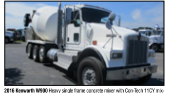
2016 Kenworth W900 Heavy single frame concrete mixer with Con-Tech 11CY mixer and 13K rear booster axle, 20K front axle, 46K full locking rears, 13K steerable lift, 248" wheelbase, Chalmers suspension, Eaton Fuller automatic transmission, rear engine PTO (REPTO), 4.78 ratio, Mixer can be removed, 20' 6" of frame behind the cab, 149" C-T, 19.263" chassis weight, 142,408 miles, sk. # 7091 - $65,500
