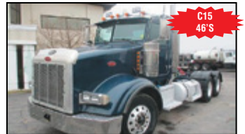
2007 PETERBILT 378: Day cab tractor with CAT C15 475hp, 18 speed manual, 12K front axle, 46K full locking rears, 203" wheelbase, Air-trac suspension, wet line, dual air cleaners and exhaust. 539,130 miles; Sk. # 7079 - $59,250
