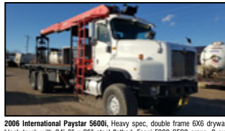
2006 International Paystar 5600I, Heavy spec, double frame 6X6 drywall/block truck with 24' 6" x 96" steel flatbed, Fassi P880 SE22 crane, 2 outriggers, 21K front axle and 46K rears, Hendrickson Haulmax suspension, 445/65R22.5 front tires and 12R24.5 rear tires, 288" wheelbase, 225" C-T, 29'8" of frame behind the cab, 5.38 ratio, and pintle hitch. Crane can be removed. 345,408 miles - $57,500
