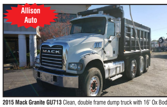
Allison Auto 2015 Mack Granite GU713 Clean, double frame dump truck with 16' Ox Bodies Inc. steel body w/ 58" sides, tarp, Mack MP7-405M engine with 405 HP engine brake, 18K front axle, 44K rears, diff. lock, 14K steerable lift axle, Allison automatic transmission, Camelback suspension, 385/65R22.5 front tires and 11R24.5 rear tires, 224" wheelbase, 136" C-T, 15" 4" of frame behind the cab. 478,177 miles, Stk# 7128 - $72,900
