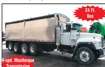
24 Ft. Box 9-spd. Maxitorque Transmission 2003 MACK RD688S, Double Frame Grain Truck w/24' Schien Equipment Aluminum Body, 6' Sides, Hoist, Roll Tarp, Barn Doors; 2 Clutches; 350 HP; 16K F/A; 44K R/A; (2) Non-steerable Lift Axles; Camelback Susp.; 315/60R22.5 Front Tires 315/60R22.5 Drive Tires; 262" WB; 178" C-T, 23" 6" Frame Behind Cab; 711,782 Miles; Stk. # 7069 - $43,000
