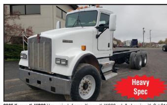
Heavy Spec 2005 Kenworth W900 Heavy single frame, Kenworth W900 cab & chassis with Cat C11 engine with 350 HP Eaton-Fuller 8LL transmission, 20K front axle, 46K full locking rears, Haulmax suspension, 425/65R22.5 front tires and 11R22.5 rear tires, 261" wheelbase, 168" C-T (muffler takes up 16"), 21" of frame behind the cab (muffler takes up 16"), 4.78 ratio, and REPTO (rear engine PTO). 143,015 miles, Stk# 4127 - $47,900
