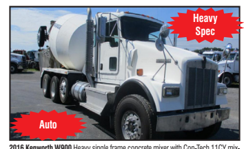
Heavy Spec 2016 Kenworth W900 Heavy single frame concrete mixer with Con-Tech 11CV mixer and 13K rear booster axle, 20K front axle, 46K full locking rears, 13K steerable lift, 248" wheelbase, Chalmers suspension, Eaton Fuller automatic transmission, rear engine PTO (REPTO), 4.78 ratio. Mixer can be removed. 20' 6" of frame behind the cab, 149" C-T, 19,263# chassis weight, 142,408 miles, stk# 7091 - $65,500
