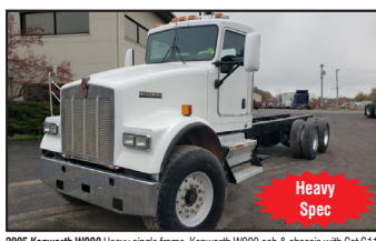
Heavy Spec 2005 Kenworth W900 Heavy single frame, Kenworth W900 cab & chassis with Cat C11 engine with 350 HP Eaton-Fuller 8LL transmission, 20K front axle, 46K full locking rears, Haulmax suspension, 425/65R22.5 front tires and 11R22.5 rear tires, 251" wheelbase, 168" C-T (muffler takes up 167", 21" of frame behind the cab (muffler takes up 167"), 4.78 ratio, and REPTO (rear engine PTO). 143,015 miles, Stk# 4127 - $47,900
