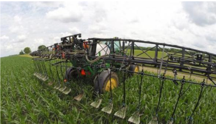
Figure 2: Side-dressing Nitrogen w/High Clearance Equipment
