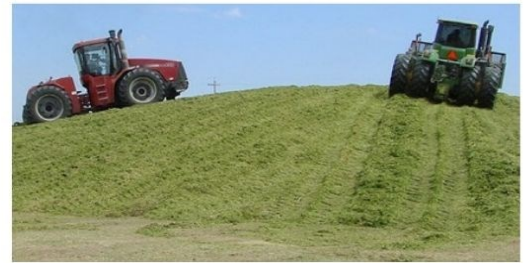
Figure 1: Two tractor operators working as a team, while packing on a safe 1 to 3 front slope in a drive-over pile.
