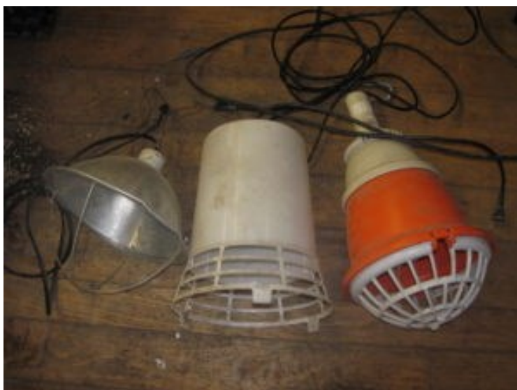
Three styles of heat lamps. Least expensive & riskiest (left) to most expensive & safest (right). Photo by Michael Glos.
