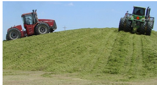
Figure 1: Two tractor operators working as a team, while packing on a safe 1 to 3 front slope in a drive-over pile.
