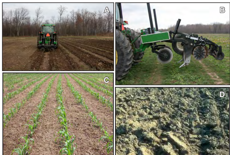
Figure 17. Examples of different tillage systems. Strip tillage with a vertical shank followed by two wavy coulters (A). Two-row strip tillage unit with an opening coulters, followed by a vertical shank, two closing coulters to form a small ridge then a rolling basket to firm the ridge (B). No-till planted sweet corn planted into a killed sweet clover fall cover crop (C). Soil following frost tillage. The large clods will mellow and break down as a result of subsequent freeze-thaw action (D).
