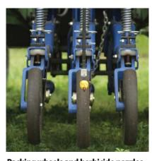
**Packing wheels and herbicide nozzles** These packing wheels ensure seed to soil contact and accurate planting depth adjustment for each of the three rows between each corn row.
