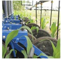
**Rear mounted spray and sidedress booms** The interseeder can apply a post emergent herbicide between rows and then sidedress fertilizer adjacent to each using this boom setup.
