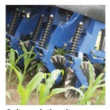
**Coulters on planting units** These coulters on each allow the interseeder to achieve good seed to soil contact in a wide range of soil and residue conditions.
