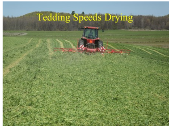
3 to 5 tons of dry matter winter forage (triticale) crops have been a challenge to dry for haylage in a day. A tedder, 2 hours after mowing, has been key to exposing lower layers to the sun.
