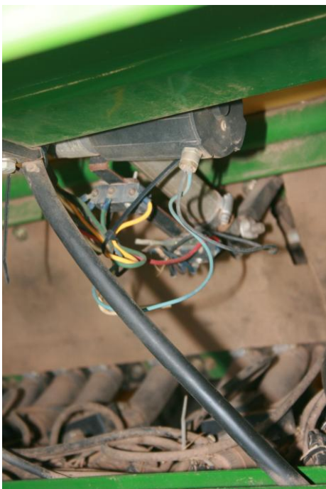
This is a photo of the linear actuator that opens and closes the door on the air seeder. The door was present on the air seeder when it was purchased.
