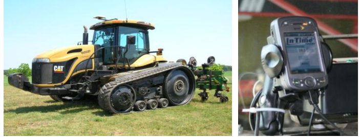
Figure 2. Tractor equipped with RTK GPS receiver and internet accessible cellular phone which receives real-time GPS correction signal from a CORS site in Lawrence County, Alabama.
